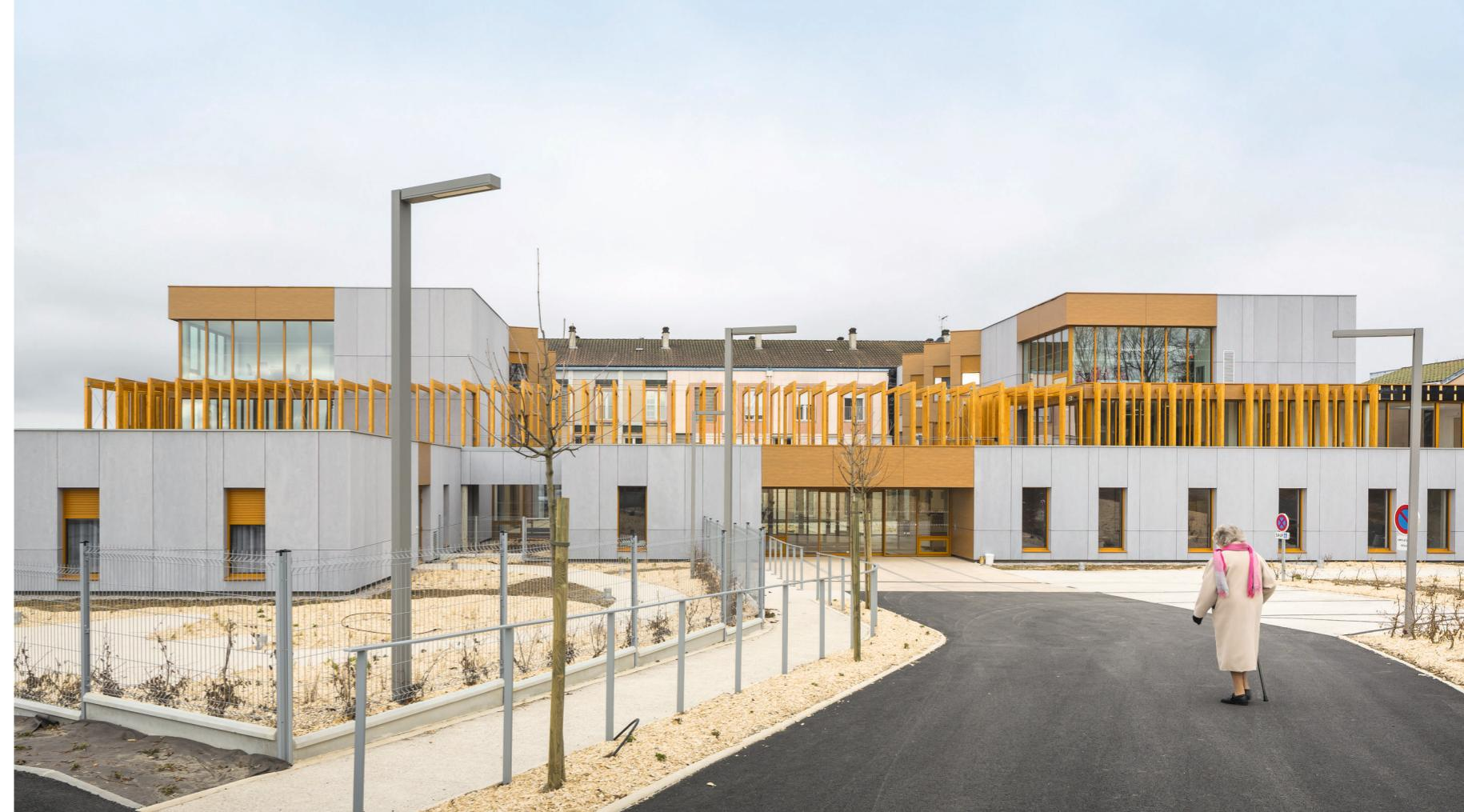
The external skin of the existing building with its gently pitched roof was also redesigned and is now made of upright light grey fibre cement panels that glow brightly in the sunlight. They are complemented by the low wood windows .
